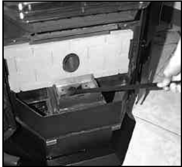
(Figure 3) - Cleaning Burn Grate
